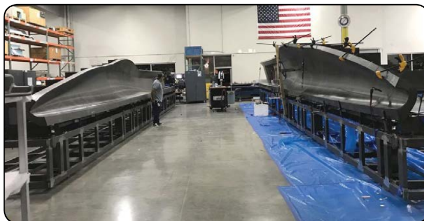
Composite layup molds for the carbon-fiber forward fuselage of the XB-1 have been completed.
