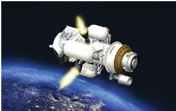
THE REDESIGNED KILL VEHICLE (PICTURED) IS DESIGNED WITH FEWER PARTS AND WIRES THAN THE CURRENT-GENERATION EXO-ATMOSPHERIC KILL VEHICLE, THEREBY BRINGING DOWN THE UNIT COST AND REDUCING THE LIKELIHOOD OF COMPONENT FAILURE. CREDIT: RAYTHEON
